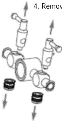
3. Unscrew the spring cap(s).
